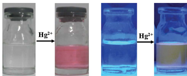
Fig. 1 Change in color (left) and fluorescence (right) of RS1 (10 \mu\text{M} ) in buffered (NaAc-HAc, pH 7.0) water–DMF (1/1, v/v) upon addition of 0.5 mM \text{Hg}^{2+} ions.
